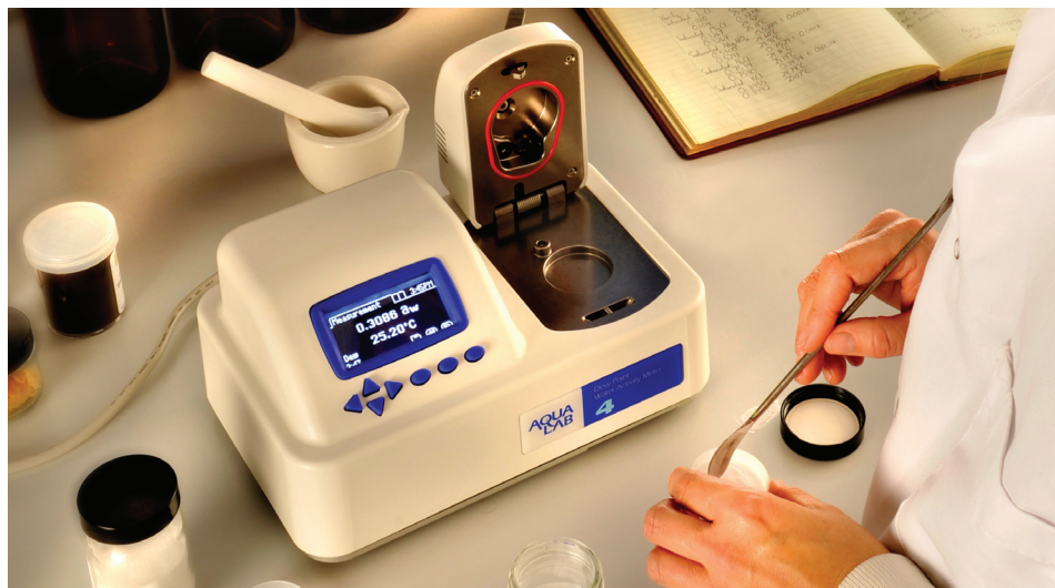
AquaLab determines water activity by measuring the temperature of the sample and the dew point of the air in a sealed head space.
