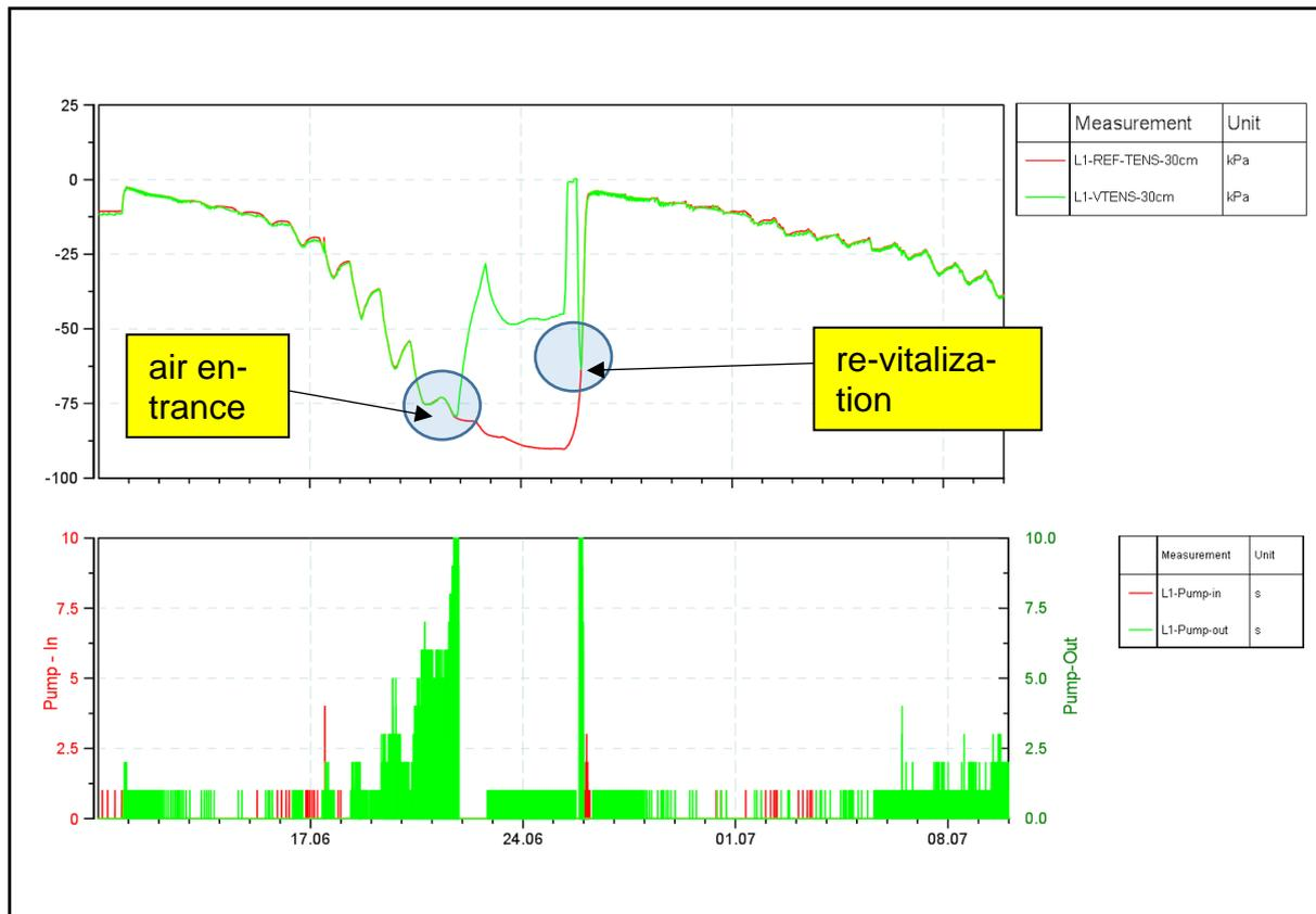
Figure 17: air entrance into the suction cup in the Lysimeter bottom
