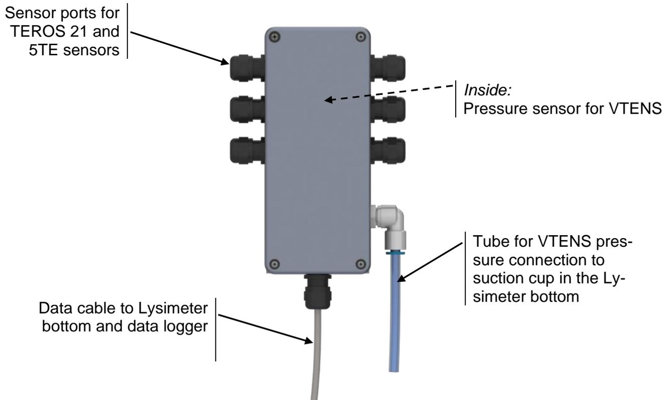
Figure 12: Lysimeter sensor distribution box
