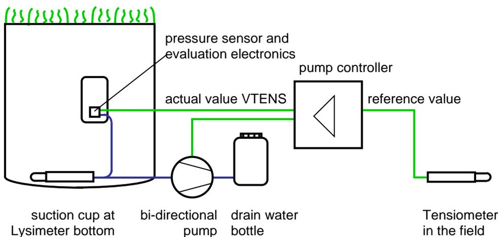
Figure 16: feedback control of the lower hydraulic boundary condition
