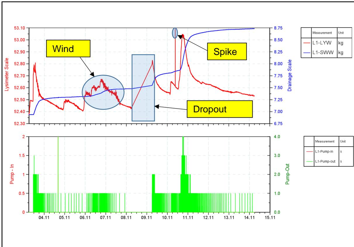
Figure 40: spikes and dropouts in measurement series
