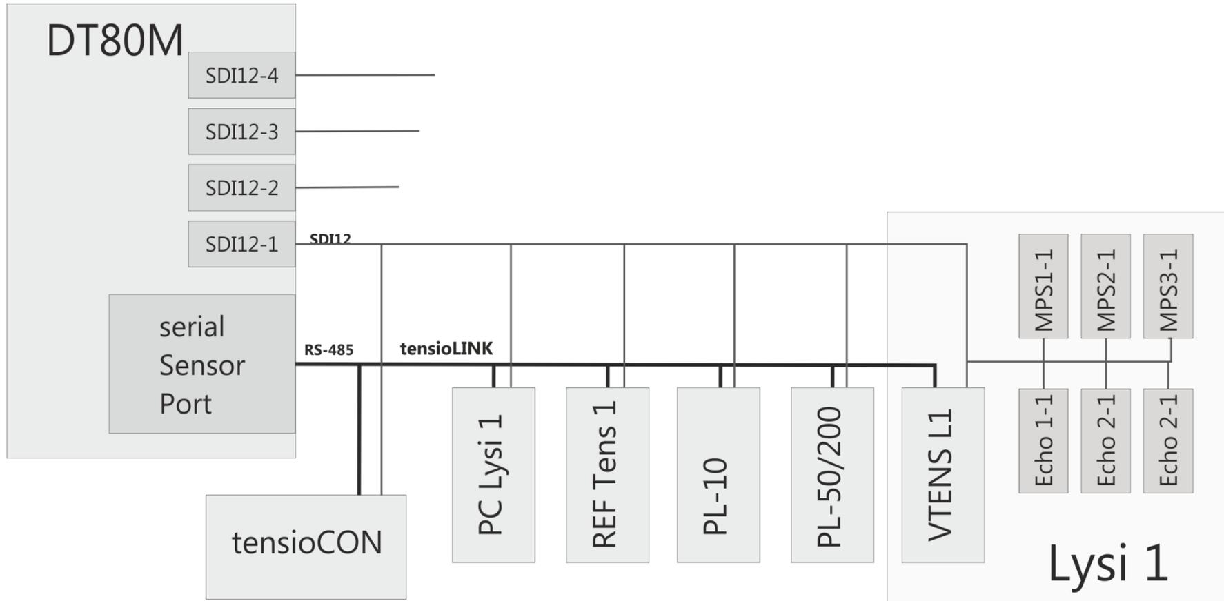
Figure 45: serial bus scheme
