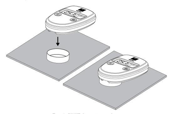
Figure 4 PAWKIT placement on sample cup
