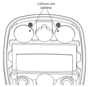
Figure 21 Lithium-ion batteries and contact springs
