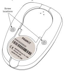
Figure 19 Battery compartment screws
