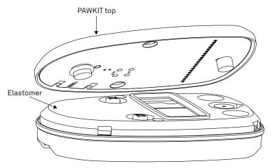
Figure 20 Separate top and elastomer
