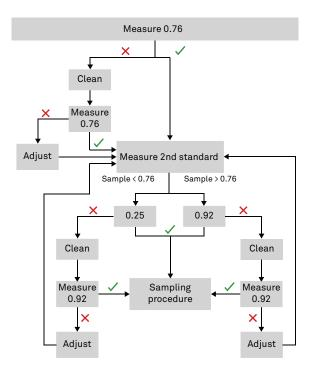
Figure 14 Calibration routine flowchart
