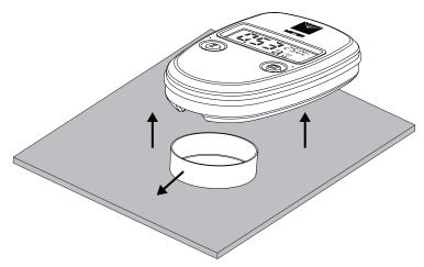
Figure 8 Remove PAWKIT when measurement complete
