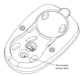
Figure 15 Thermopile sensor lens
