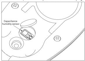
Figure 17 Capacitance humidity sensor
