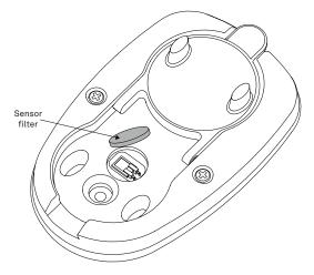
Figure 16 Filter removal
