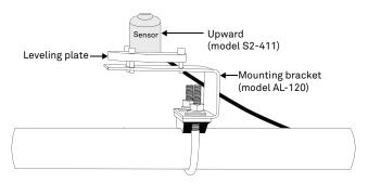
Figure 2 Upward-facing sensor installed on mounting post
