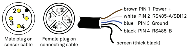
Figure 6 4-pin M12 plug wiring
