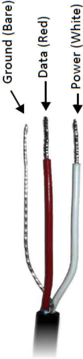
Figure 2: Pigtail End Wiring
