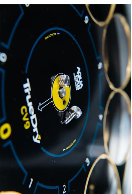
Figure 28: Removing Thumb Screws
