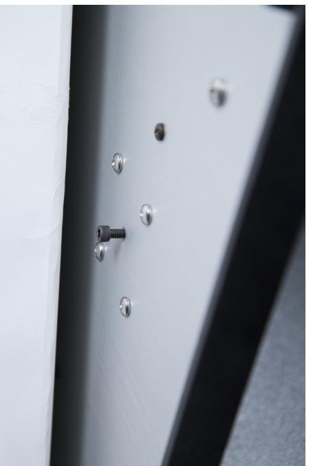
Figure 6: Loosened Shipping Screw
