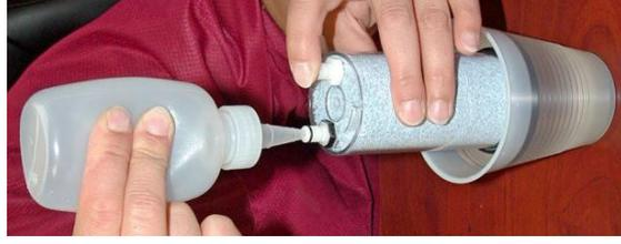
Figure 33: Checking Desiccant Cartridge for Leaks
