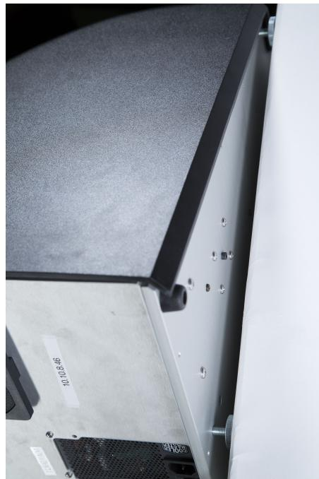
Figure 5: Locate Shipping Screw
