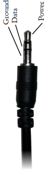
Figure 1: 3.5 mm Stereo Plug
