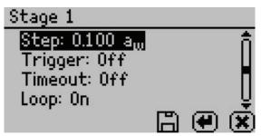
Figure 45 Selecting Stage 1 step interval
