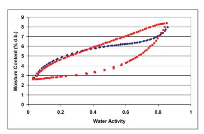
Figure 23 Working and full isotherm for wood pulp
