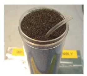
Figure 25 Desiccant cartridge foam
