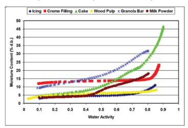
Figure 19 Moisture adsorption isotherms
