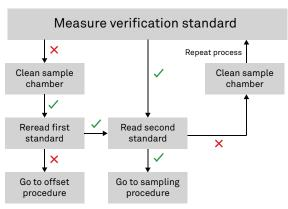
Figure 29 Verification standard flowchart. A check indicates AQUALAB VSA verified the standard within specification; a cross indicates AQUALAB VSA did not verify the standard within specifications.
