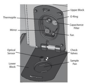
Figure 28 AQUALAB VSA sample chamber diagram
