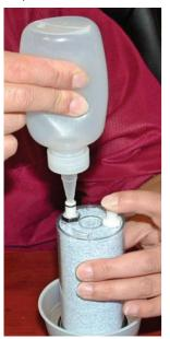
Figure 27 Checking desiccant for leaks
