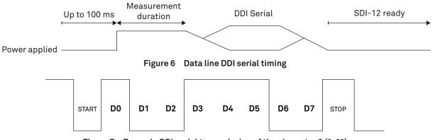
Figure 7 Example DDI serial transmission of the character 9 (0x39)
