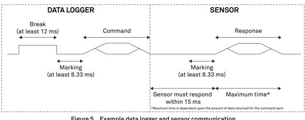
Figure 5 Example data logger and sensor communication
