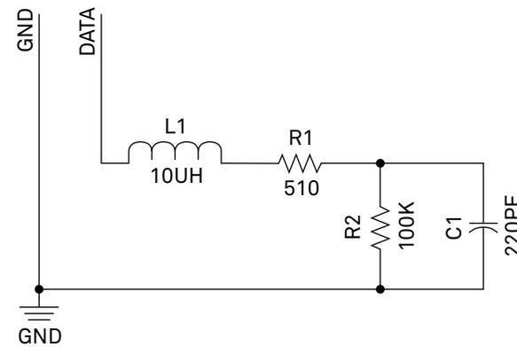
NOTE: This is a low-impedance variant of the recommended SDI-12 specification. This allows as many as 62 sensors to be maintained on a bus.
