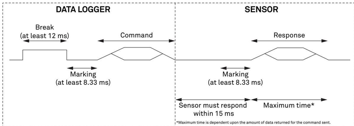
**Figure 5 Example data logger and sensor communication**
