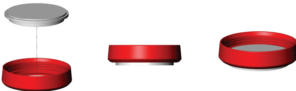
Figure 1 Figure 1 Assembly of the KSAT bottom gasket
