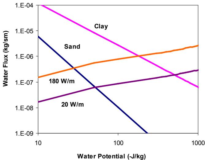
Figure 1. Graph of eq. 4 and eq. 10 for sand and clay liquid flow estimates, and high and low heat dissipation rates.
