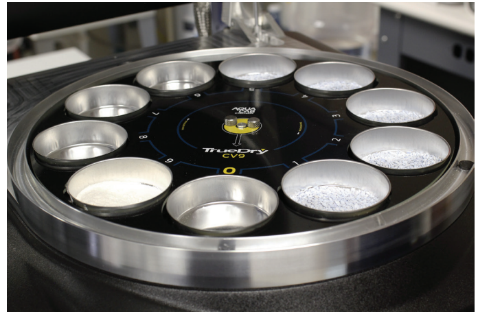
Figure 1. Turntable design of the TrueDry to enable analysis of 9 samples simultaneously.
