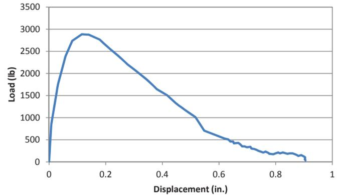
Figure 6. Load - displacement plot for Sample 1 (vertical orientation).
