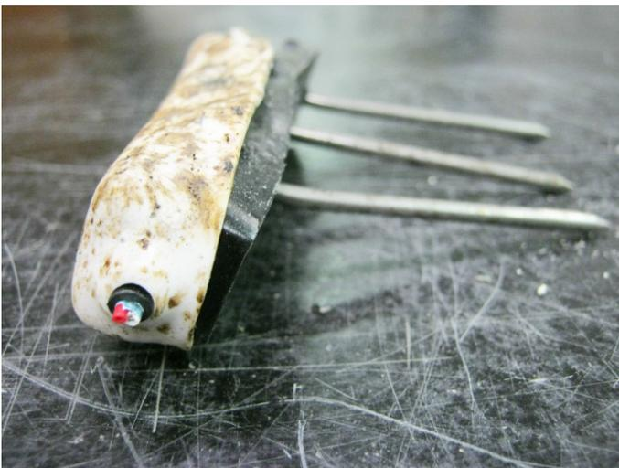
Figure 11. Sensor 2 after compression testing (horizontal orientation).
