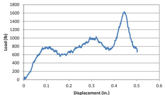
Figure 8. Load - displacement plot for Sensor 1 (vertical orientation).
