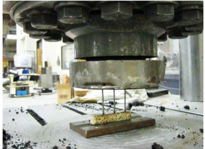
Figure 4. Sensor 1 in compression machine.
