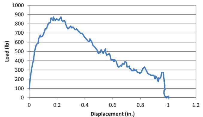
Figure 7. Load - displacement plot for Sample 2 (horizontal orientation).
