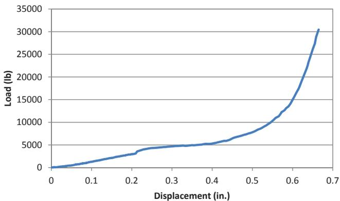
Figure 10. Load - displacement plot for Sensor 2 (horizontal orientation).
