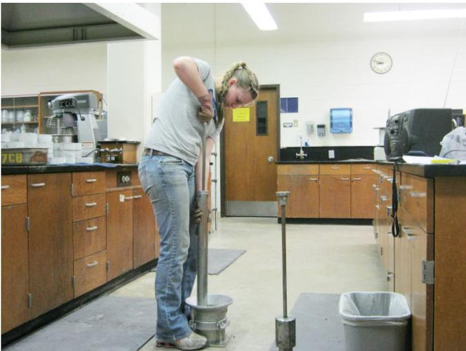
Figure 1. Asphalt sample compaction using a modified Proctor hammer.
