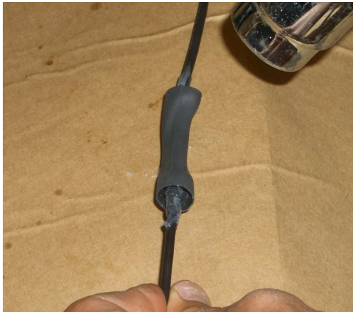
Figure 6 – Heat shrink tubing with silicone over the entire connection (A); the final product (B).
