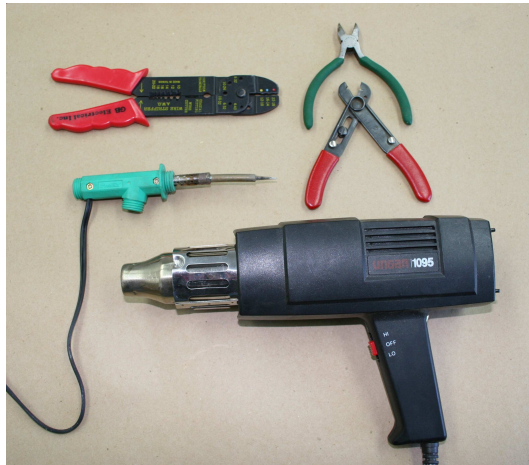
Figure 1 – Wire strippers, wire cutters, soldering iron, heat gun (A), heat shrink tubing, rosin-core solder, flux paste, and silicone rubber sealant used for wire splicing (B).
